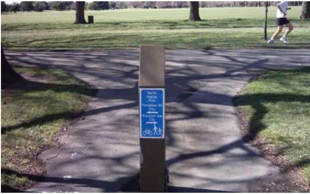
**Figure 12: Good directional signposting, but far too small to be read while moving at normal cycling speed**
